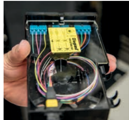
MPO optical fibre cassette, custom made by Legrand. Installation time cut in half in comparison with the old system that was in use.
